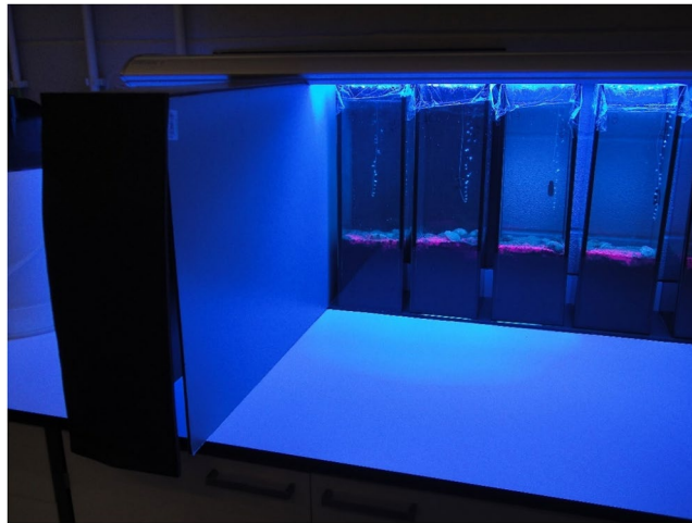
Figure 4. Particle reworking was measured inside a black box, photographing the pink luminophores exposed to four actinic lights 22000 K Rede-sea 80 W ( \lambda = 400\text{--}450\text{ nm} ).
