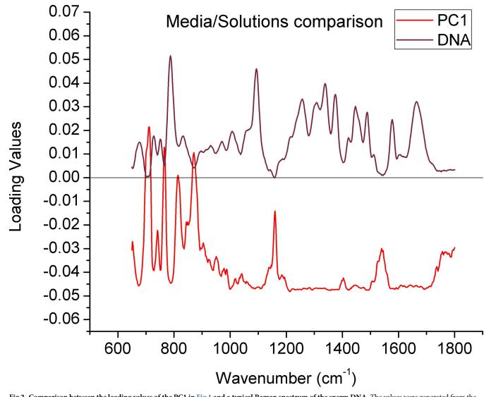
Fig 2. Comparison between the loading values of the PC1 in Fig 1 and a typical Raman spectrum of the sperm DNA. The values were generated from the comparison of the different media/solutions. The black line denotes zero in the loading values.
