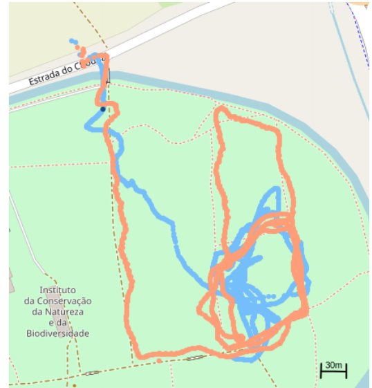
Figure 4.2: GNSS test results. Position tracking of the Xiaomi Mi 9T and the Xiaomi Mi Mix 3 is displayed in blue and orange, respectively.
