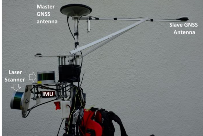
Figure 2.10: Backpack apparatus for dataset collection presented by Oveland et al. [42].
