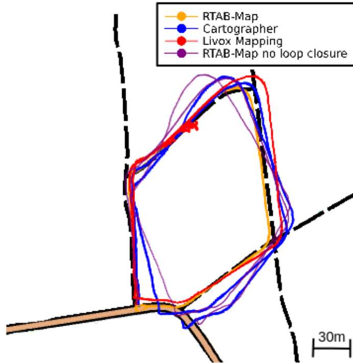
Figure 5.10: Overlaying the path generated by the SLAM on the map adapted from [58].
