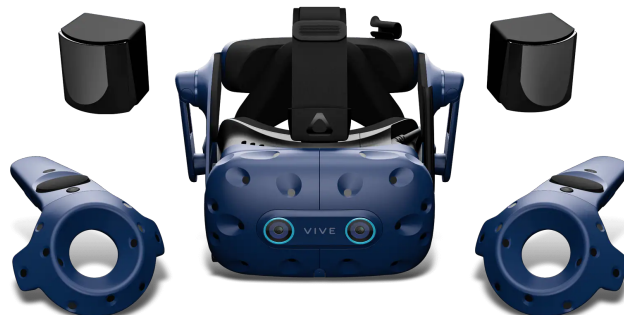
Figure 3.3: HTC Vive Pro Eye VR system, the Head Mounted Display (HMD) in the centre, the two lighthouses in the back and the two controllers in front.
