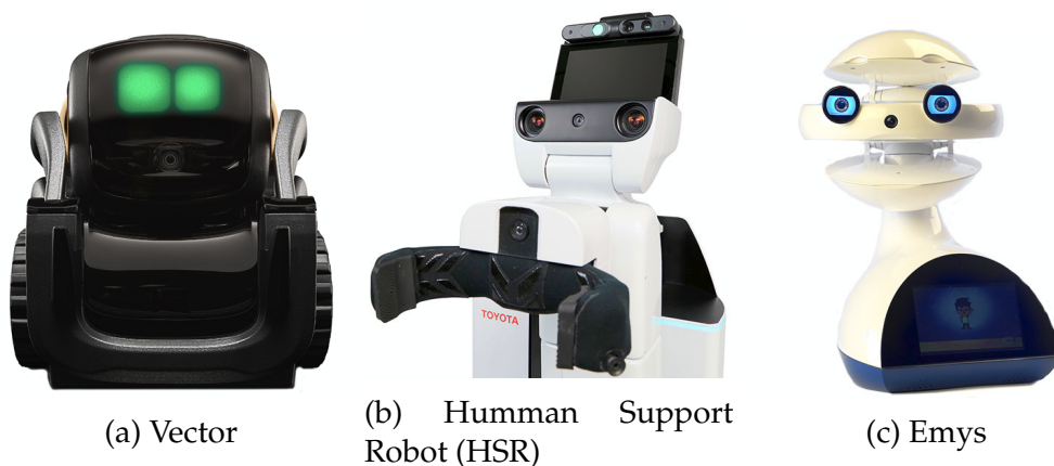
Figure 2.5: Different types of consumer service robots. Vector (a) is used as a companion robot; HSR (b) is used to watch family members and fetch objects; Emys (c) is used in education to teach foreign languages to kids.
