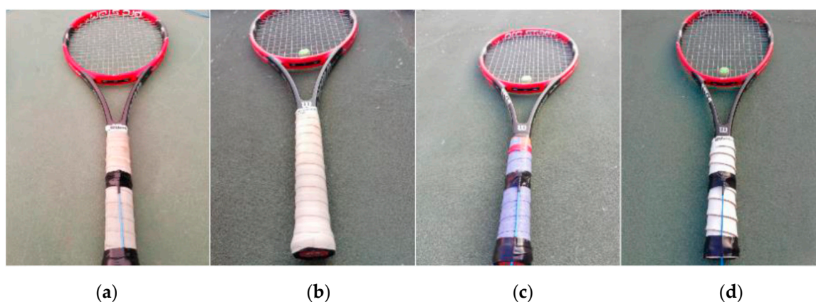
Figure 1. Racket grip test conditions: (a) Wilson Pro with without anti-vibrator (WGNV); (b) Wilson Pro with an anti-vibrator (WGWAV); (c) Wilson Pro with Tourna and anti-vibrator (TGWAV); (d) Wilson Pro with Corck and anti-vibrator CGWAV.
