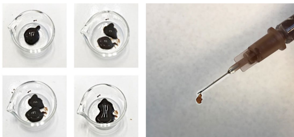
Figure 3.7. Macroscopical evaluation of hydrogels. (left) - self-healing ability of the PS1-PEG-CS hydrogel within 1 hour observation, (right) - injectable properties of PS3-PEG-CS hydrogel.
