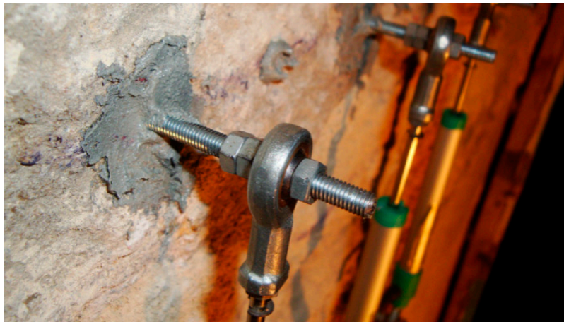
Figure 12. Displacement transducers attached to the wall.
