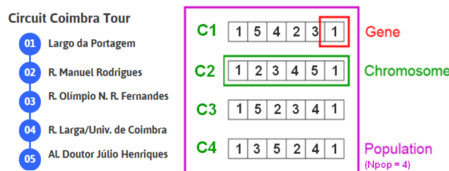
Figure 7. Example of a population of the genetic algorithm, for the problem of visiting five different places. The population contains four individuals, each individual consisting of five genes—one for each location.
