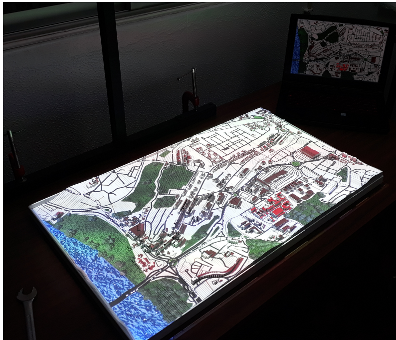
Figure 6. Physical model, with the projection of the city model over the wooden structure and showing the computer screen behind for comparison.
