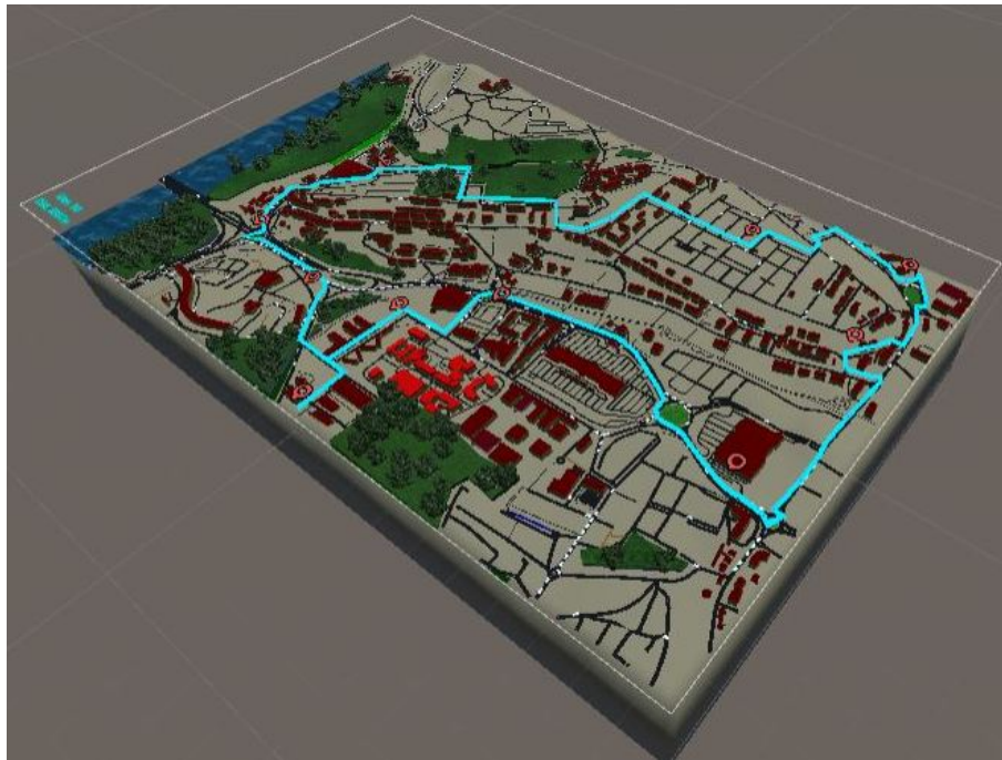
Figure 10. Example of a path planned to visit ten different points of interest, simulated in the computer. The red donuts are points of interest, the solution path is marked in blue.
