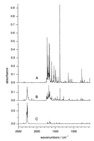
Figure 6. Infrared spectrum of (A) 1-methylcytosine isolated in an Ar matrix recorded immediately after deposition, (B) 1-methylcytosine isolated in an Ar matrix after 2 h of UV ( $\lambda$  > 295 nm) irradiation, and (C) UV-irradiated (1 h,  $\lambda > 320$  nm) 1-methyl-2(1*H*)-pyrimidinone.
