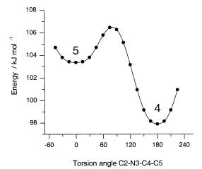
**Figure 5.** MP2/6-31++G(d,p) calculated potential energy curve for interconversion between forms **4** and **5** of the open-ring conjugated isocyanate. Each point was calculated by fixing the value of the torsional angle C2-N3-C4-C5 and optimizing all other parameters defining the geometry of the system. Energy of the closed-ring form was chosen as the reference (zero relative energy) level.
