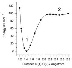
Figure 3. MP2/6-31++G(d,p) calculated potential energy curve for conversion from the open-ring form 2 to the closed-ring structure of 1-methyl-2(1H)-pyrimidinone (deep minimum at 1.42 Å). Each point was calculated by fixing the value of the distance between atoms N1 and C2 and optimizing all other parameters defining the geometry of the system. The calculated energy at the closed-ring minimum was -377.790 753 6 hartree.
