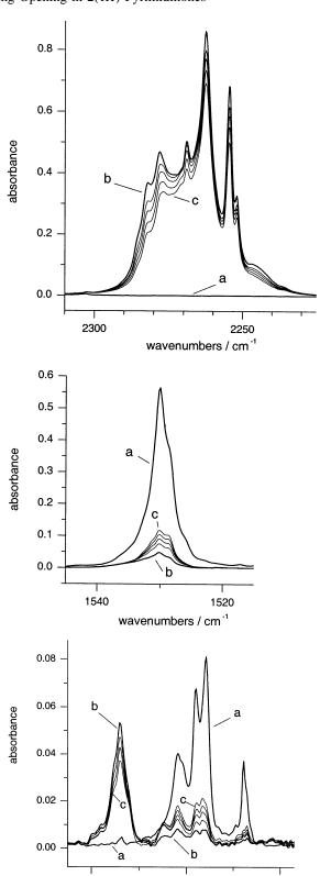
Figure 2. Portions of the infrared spectrum of 1-methyl-2(1H)pyrimidinone isolated in an Ar matrix: (a) after deposition of the matrix; (b) after 1 h of UV ( $\lambda > 320$  nm) irradiation; (c) after subsequent 16 min of UV ( $\lambda$  > 270 nm) irradiation. Traces between traces b and c present the progress of the UV ( $\lambda > 270$  nm)-induced photoreaction and correspond to irradiation times of 2, 4, and 8 min.
