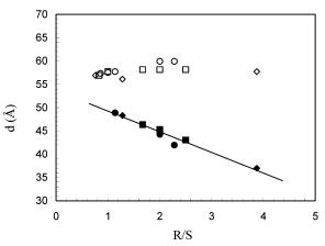
**Figure 9.** Repeat distances, taken from SAXS diffractograms in Figure 8a, for the DNA–DNA spacing,  $d_{\text{DNA}}$  (filled symbols), and the interlayer distance,  $d_{\text{mem}}$  (open symbols), as a function of the concentration ratios, [DNA]/[S<sup>+</sup>], D/S. Different symbols correspond to different net surfactant charge concentrations: (**■**), [S<sup>+</sup>] = 1.2 mM; (**♦**), [S<sup>+</sup>] = 2.3 mM; (**●**), [S<sup>+</sup>] = 3.5 mM.
