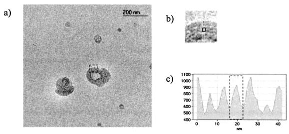
**Figure 7.** Multilamellar structures formed by the interaction of DNA with catanionic vesicles. (a) Cryo-TEM image of DNA-vesicle complexes;  $[DNA] = 2.88 \text{ mM}, [S^+] = 2.22 \text{ mM}; D/S = 1.30$ . (b) Magnified detail of the lamellae details from (a). (c) Line profile with an integration-area width given by the area shown in (b).
