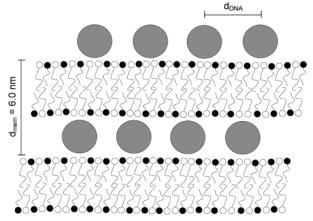
**Figure 10.** Schematic representation of the proposed structure for DNA-catanionic vesicle complexes.
