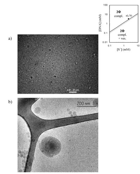
Figure 6. Light (a) and cryo-TEM (b) images for  $[S^+] = 2.22$  mM and [DNA] = 2.88 mM. Only DNA-vesicle complexes are present in solution.
