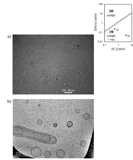
**Figure 4.** Light and cryo-TEM micrographs for solutions in the aqueous DNA–CTAB/SOS system: (a)  $[S^+] = 0.62 \text{ mM}$  and [DNA] = 0.25 mM, a small number of vesicles in coexistence with complexes; (b)  $[S^+] = 3.77 \text{ mM}$  and [DNA] = 0.05 mM, vesicles in coexistence with a few DNA–vesicle complexes.
