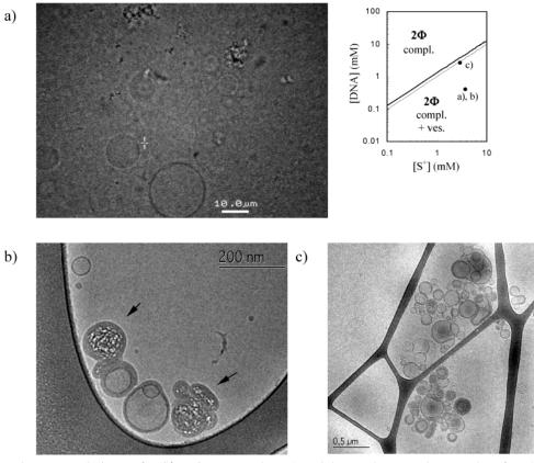
**Figure 5.** Light (a) and cryo-TEM (b) images for  $[S^+] = 3.77$  mM and [DNA] = 0.4 mM. There are a large number of DNA-vesicle complexes in coexistence with unperturbed vesicles and also some complex aggregates. (c) Cryo-TEM images for  $[S^+] = 2.89$  mM and [DNA] = 2.80 mM, showing aggregates of complexes in coexistence with vesicles. Arrows denote beam-damaged material.
