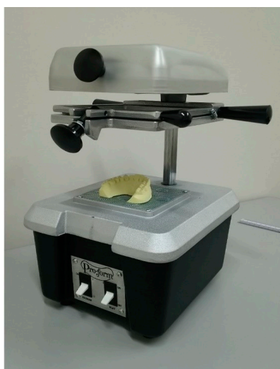
Figure 10. Typical vacuum forming machine (adapted) [54]. Copyright Wiley-VCH Verlag GmbH & Co. KGaA. Reproduced with permission.
