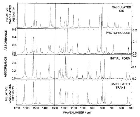
**Figure 5.** Comparison of the experimental IR spectra of the substrate and the photoproduct with the calculated spectra (at the DFT(B3LYP)/6- $31G^{**}$  level) for the trans and cis isomers of DMACS. Note the change of the ordinate scale at 1300 cm<sup>-1</sup>. The calculated frequencies are scaled with a uniform scale factor 0.97.
