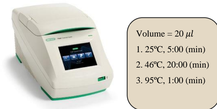
Figure 16. PCR T100 Thermal Cycler (Bio-Rad Laboratories, California, USA) and protocol of cDNA conversion.
