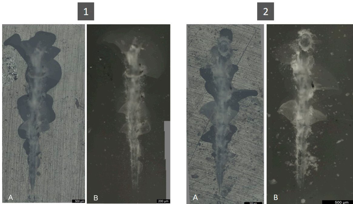
Figure 9. Observation of wear suffered by a specimen of the control group (1) and test group (2): (A) Non-polarized lens; (B) Polarized lens.
