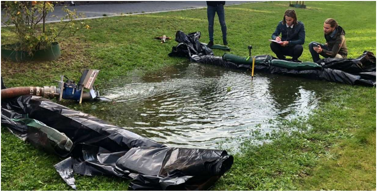
Figure 4.3 - View of the swale infiltration test that was carried out in Paddepoel in Groningen, The Netherlands (Source: ClimateScan)
