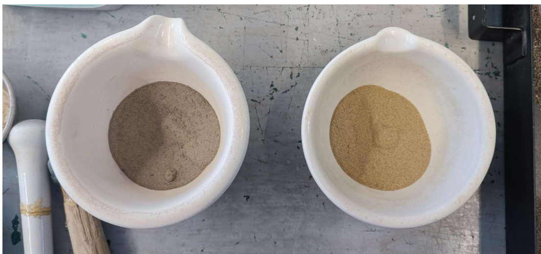
Figure 3.13 - Disintegration of the soil samples using mortars
