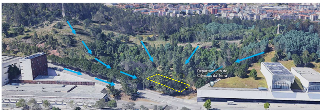
Figure 5.5 - Draw illustrating the location of the swale and drainage area (Source: Google earth), in Campus II of the University of Coimbra.
