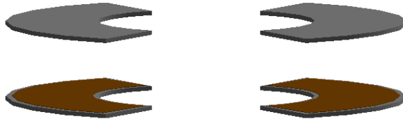
Figure 5.1: Simulation detector: upper and lower bases. In gray, the ABS plastic; in brown, the copper plates.
