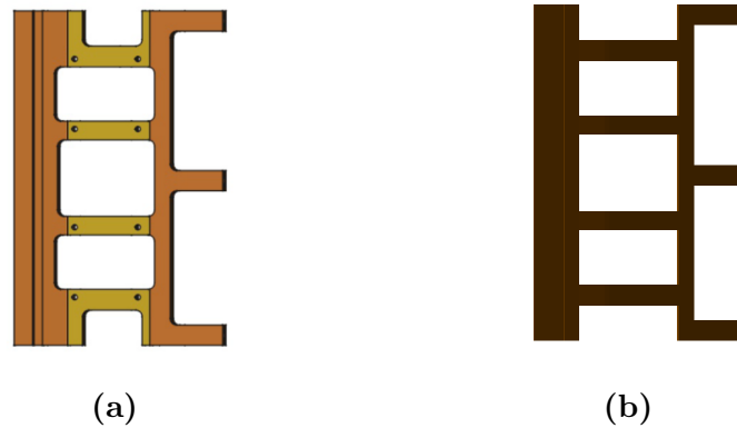
Figure 5.8: Lateral view of the ribs. The geometrical approximations made from the prototype rib (a) to the one developed in the G4VSolid approach (b) are perceptible.
