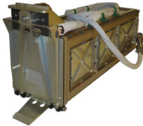
Figure 2.12: P-POD MkIII REV E, image from [15]
