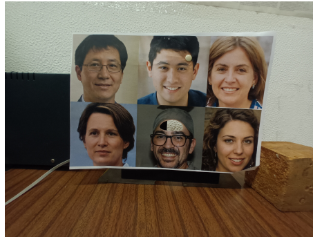
Figure 4.10: Six-faces scene - the face on the middle bottom position has a hole on the forehead position, where the heatsink will be placed, in order to simulate a high temperature for the forehead.
