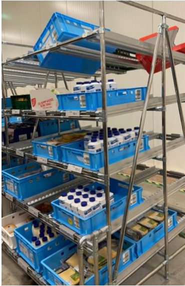
Figure 4.4 Flow Rack Storage System in FC2
