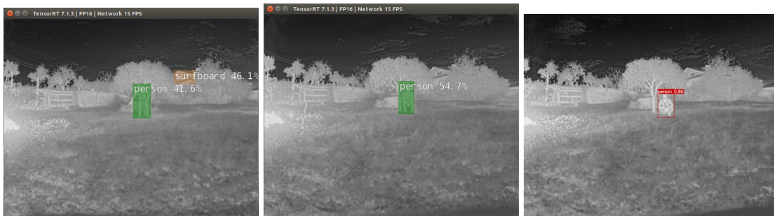
(a) SSD Mobilenet V2, with a (b) SSD Mobilenet V2, with (c) YOLOv7, with a 86.0% of 41.6% of confidence for 25% a 54.7% of confidence for confidence for 50% threshold. 50% threshold. old.
