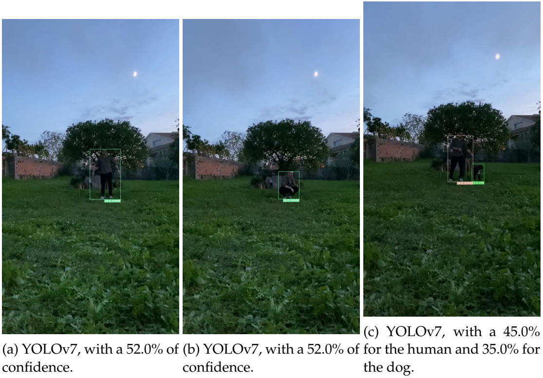
Figure 4.26: YOLOv7 detection at 9 meters.
