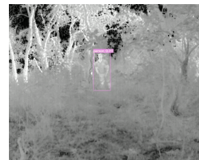
(b) YOLOv7, with a 71.0% of detection confidence for the human.
