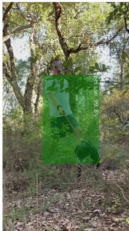
(a) SSD Mobilenet V2, with 99.8% hu- man detection confidence.
