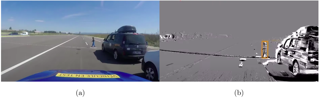
Figure 3.2: Comparison between the output from traditional frame cameras (a) and DVS (b) when in a real context. (Taken from https://youtu.be/MjX3z-6n3iA )
