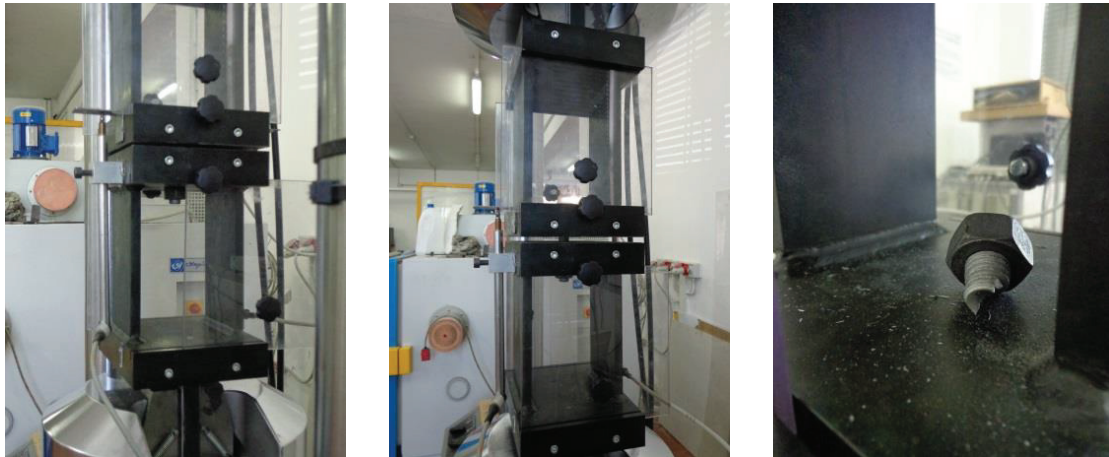
Figure 5.9: Monotonic test of the M16 HR Cl. 10.9 assembly at different stages
