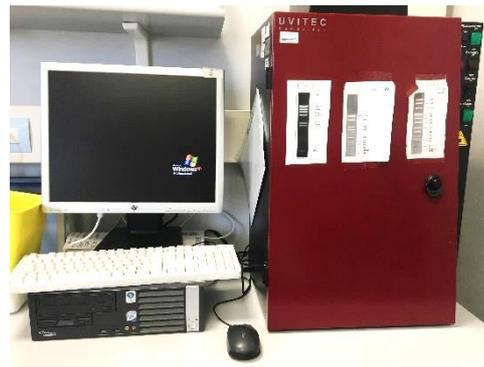
**Figure 11** - UVITEC Cambridge equipment for the visualization record of the agarose gel
