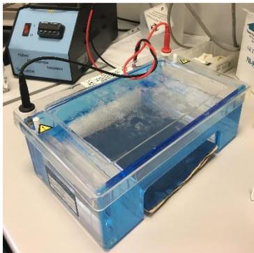
**Figure 10** - Gel box immersed with a buffer, with a positive and negative power source.
