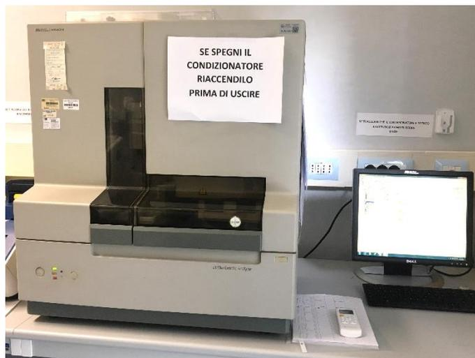
**Figure 16** – Genetic Analyzer from Applied Biosystems; Equipment for genetic sequencing and analysis of DNA fragments
