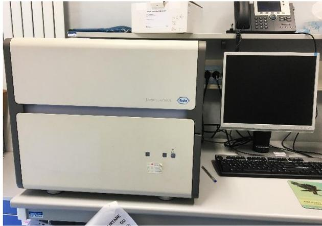
**Figure 13** - Station for performing Quantitative Real-Time PCR; LightCycler 480 Instrument II from Roche performs the Real-Time reaction, and data is visualized on the computer.
