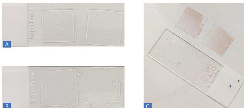
Figure 8 - Formation of gels and coverslips removal. A- Menzel Gläser SuperFrost® microscope coverslips (Thermo Fisher Scientific) showing intact gels; B- HistoStar™ (Vidrolab) coverslips compromising the integrity of the gels; C- Coverslips from HistoStar™ (Vidrolab) – examples where gels did not adhere to the slide.
