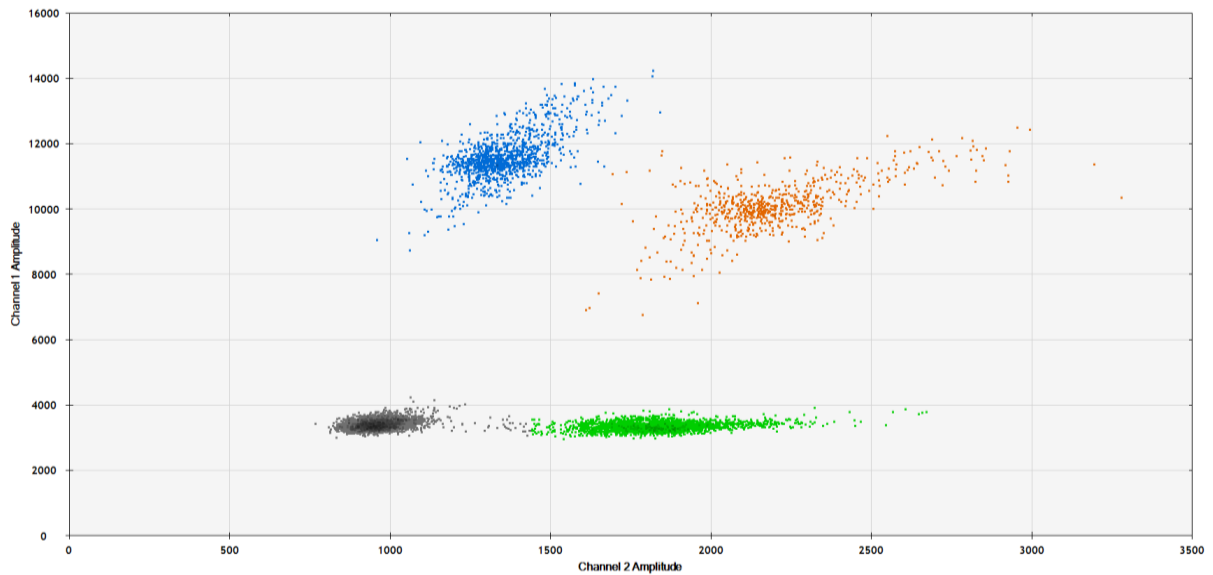
Figure 4 Representative 2D scatter plot of a ddPCR result. Groups are automatically assigned into distinct areas (clusters) by the software, with the blue cluster representing the probe of interest, the green cluster the RPP30 probe, the black cluster the negative droplets and the orange clusters representing the droplets with both probes present.
