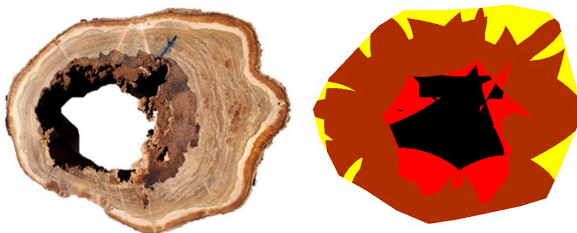
Figure 4. Example of ultrasound tomography image. Source: Reproduced with permission from Raquel Gonçalves (2021), Nondestructive Testing Research Group Coordinator, School of Agricultural Engineering, University of Campinas, Brazil. Legend: Yellow = velocities from 80% to 100% of maximum velocity; Brown = velocities from 50% to 80% of maximum velocity; Red = velocities from 36% to 50% of maximum velocity; Yellow = velocities from 0% to 36% of maximum velocity.
