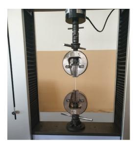
tested at both filament (100 mm segments) and printed specimen (100 mm  $\times$  20 mm  $\times$  2 mm, according to ASTM D3039) configurations. Figure 2 shows a representative filament test.
