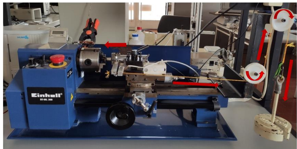
Figure 4. Pin-on-Disc Tribometer used in tribological tests (the red arrows indicate the direction of application of the force).
