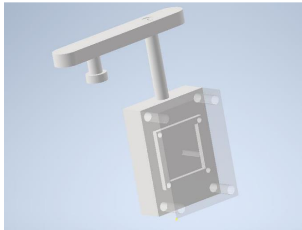
Figure 30. 3D design of the proposed sample holder.
