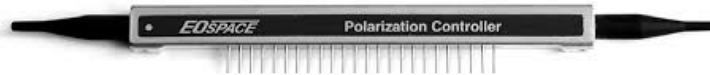
Figure 3.1: Image of the actual EOSPACE Polarization Controller with the pins to apply voltages on the bottom. Each sequence of 3 pins is linked to one stage
