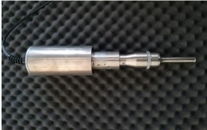
Figure 8. Transducer connected with the ultrasonic horn.
