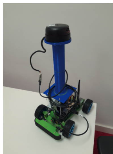
Figure 3.4: 3D printed the second prototype.
