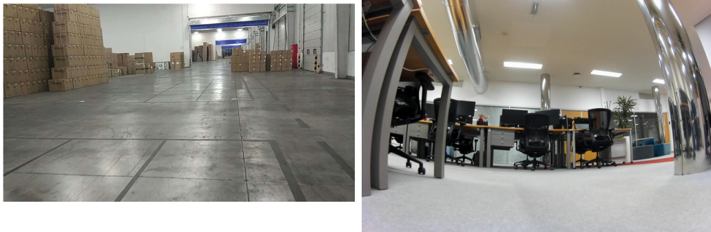
Figure 7.4: Left: In the test environment of the article, [21], Google Cartographer algorithm was able to achieve an average error of less than 10 cm. However, we must point out that the environment does not contain reflective or transparent surfaces and is more simple. Right: As we can observe, the CSW text environment is much more complex, with lots of chairs, tables, and reflective and transparent surfaces.
