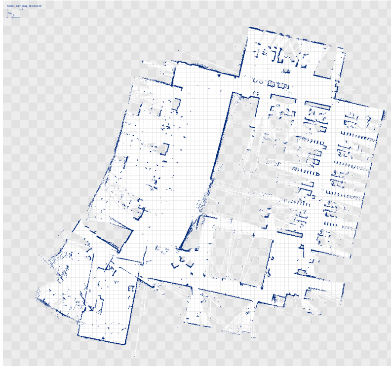
Figure 3.5: Critical Software Coimbra Office B, first floor. Image generated by Hector SLAM in our robotic agent.
