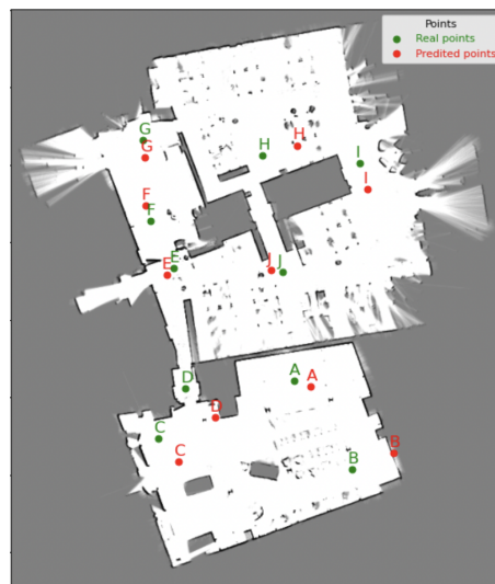
Figure 7.2: Best results obtained with old LIDAR device - average error of 1.622 m and a variance of 0.590 m.
