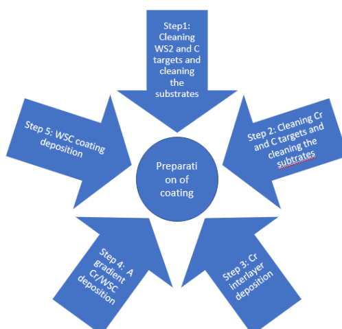
Figure 3.1. Illustration of coating preparation
