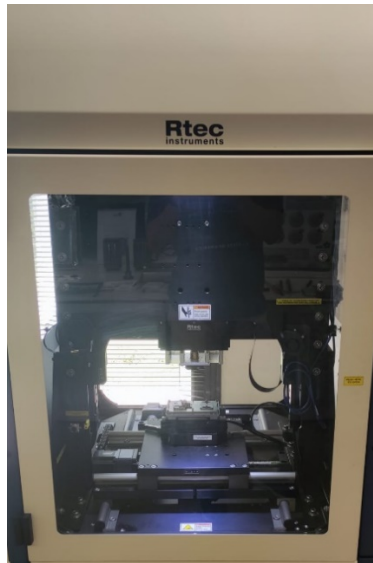
Figure 3.3. Rtec universal tribometer machine equipped with optical microscope
