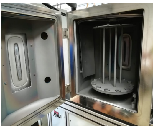
Figure 3.2. A sputtering magnetron instruments
