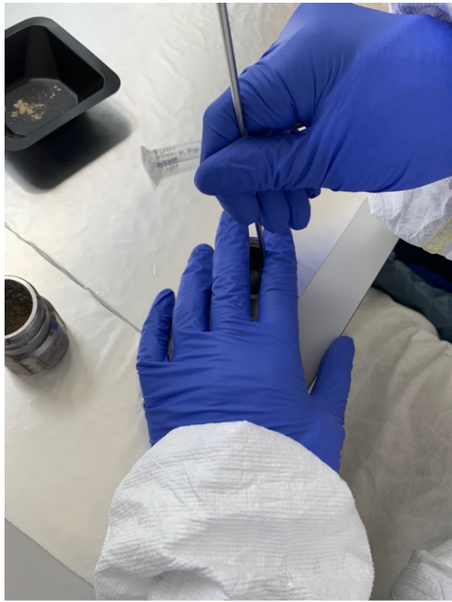
Figure 12 When the milling process is finished, remove the jar from the mixer mill. Carefully open the jar and roughly scrape off the upper part with a clean spatula. Collect the powder in the boat. Then carefully drop the ball that was previously in the lower part into the upper part of the jar and try to get as much powder off the ball as possible.
