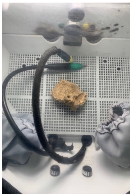
Figure 6 Before the grinding process can start put the sample into a cross-linker for a total of 10 minutes on each side. Then, switch on the sandblaster and plugged in vacuum cleaner on and place the sample into the cleaned grinding hood.
