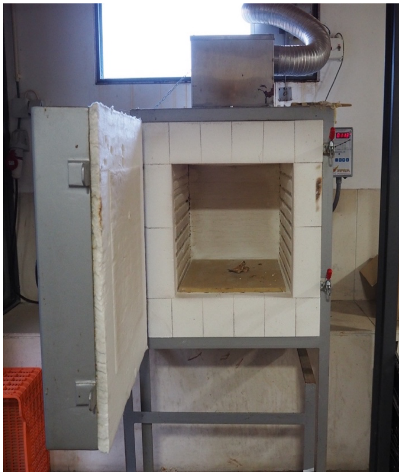
Figure 4 Electric muffle furnace with thermostat at the Faculty of Life Sciences of the University of Coimbra. The bones were placed in the oven with the inner acoustic meatus facing upwards, as shown in the picture.
