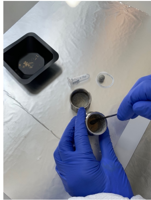
Figure 13 Pour most of the powder that is in the lower part of the jar into the boat and scrape the lower part thoroughly. Weigh the powder and store it in a DNA low bind tube in the refrigerator.
