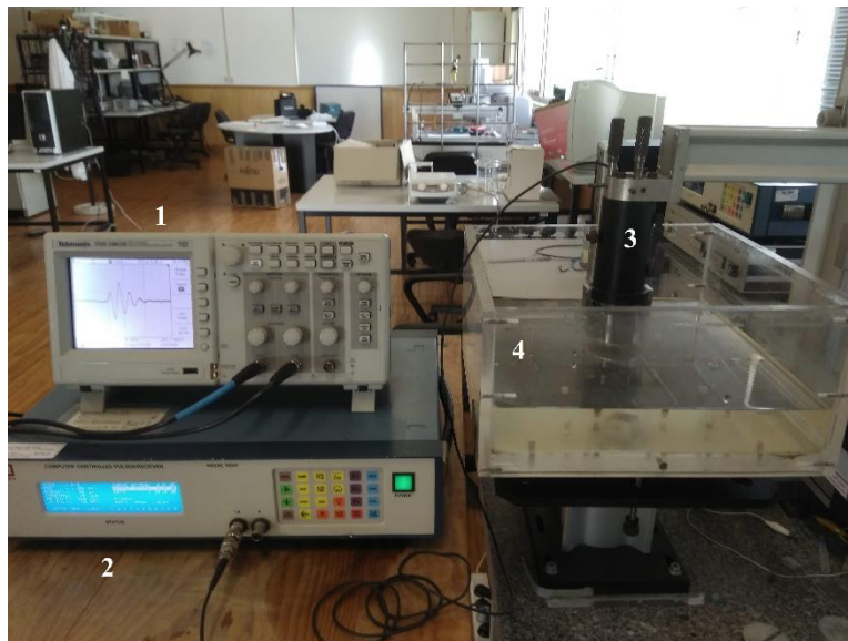
Figure 5.2. Experimental setup: 1) oscilloscope, 2) pulser/receiver, 3) micro positioning system, 4) acrylic container.
