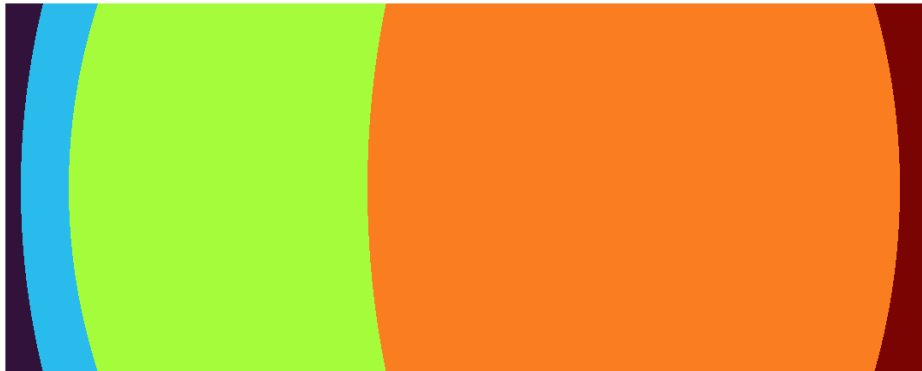
Figure 4.22. Central slide of the 3D eye matrix with a pixel size of 8 \mu\text{m} . Components: water (black), cornea (blue), aqueous humor (green), lens (orange), and vitreous humor (red).
