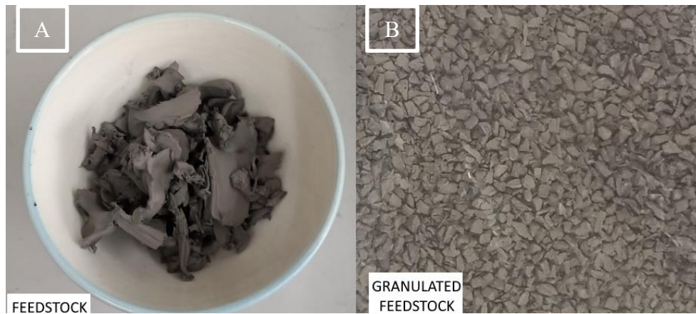
Figure 4.2. Feedstock A) after mixing, and B) after granulation.
