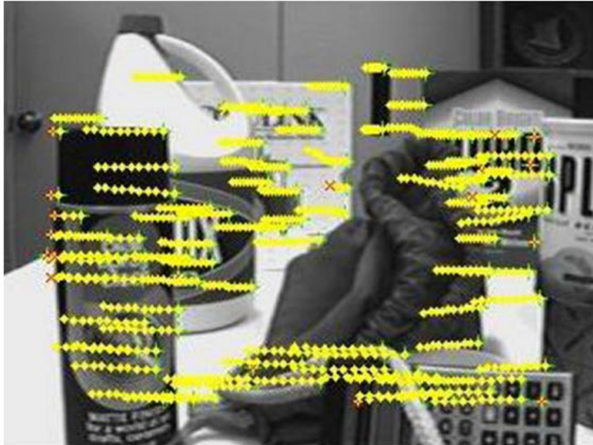
Fig. 1.2 Tracking and integration of the various features present in each of the images of the frame sequence. (Image from: [1])
