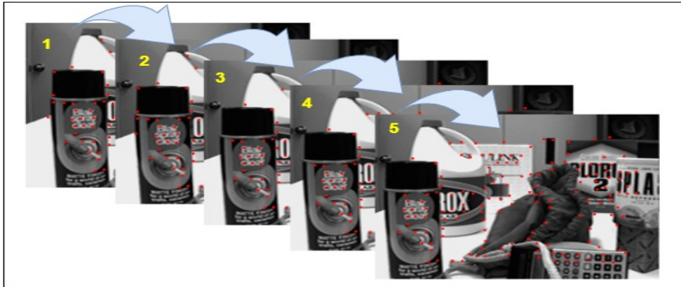
Fig. 1.1 Example of tracking performed with KLT. The images contain the detected features in a sequence of frames.
