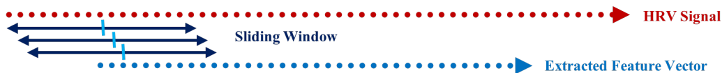
Figure 5.2: Schematic representation of the extraction of a feature using one of the sliding windows. In the end we obtain a total of 558 feature vectors, corresponding to the 31 features times 18 window sizes, for each experiment run.
