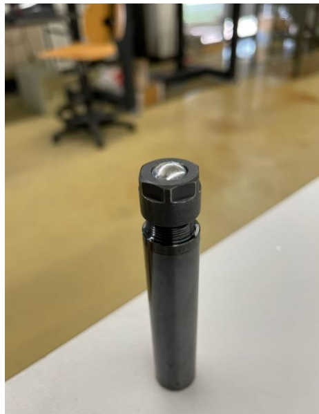
Figure 3.8: Aluminium Ball used as a counter body on the holder.
