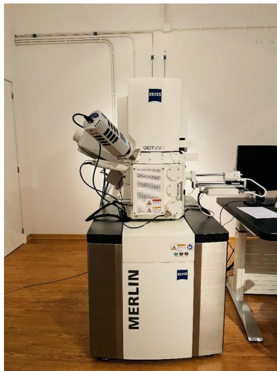
Figure 3.3: The SEM instrument equipped with WDS detector used for studying morphology and chemical analysis of the film.
