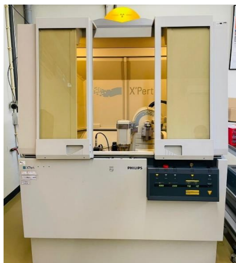
Figure 3.5: XRD setup for the experiment.
