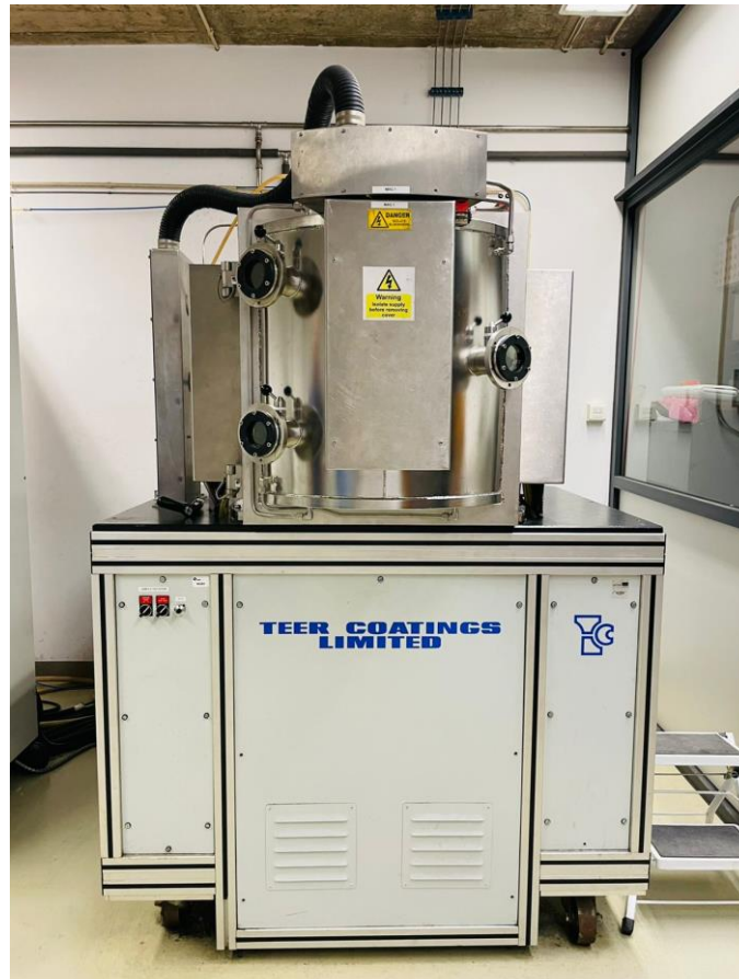
Figure 3.2: Deposition unit setup coatings.
