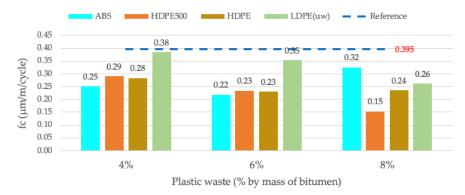
**Figure 14.** Results for the accumulated strain (ε3600) and creep rate (*fc*).
