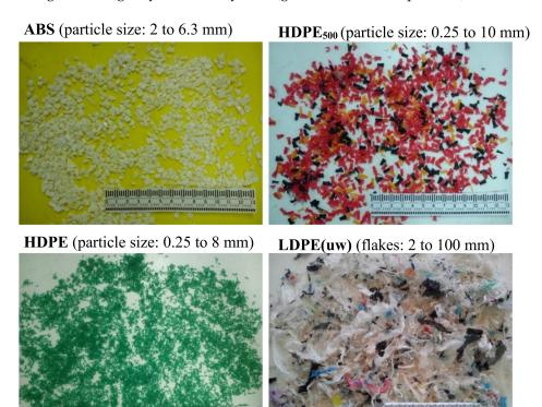
Figure 2. Types of plastic waste used as polymers in the studied asphalt mixtures in the present study.
