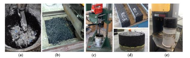
**Figure 4.** View of the mixing procedure and production of specimens: (**a**) incorporation of plastic waste by the dry process; (**b**) compaction of slabs with a tandem roller; (**c**) compaction of cylindrical specimens with a vibrating hammer; (**d**) prismatic and cylindrical specimens to mechanical performance evaluation; (**e**) gyratory compactor and cylindrical specimen moulded.
