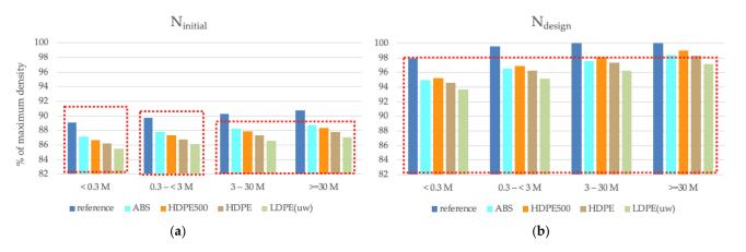
**Figure 15.** Comparison of the workability measured in gyratory compaction tests with the SUPER-PAVE limits for (**a**) N<sub>initial</sub> and (**b**) N<sub>design</sub>.
