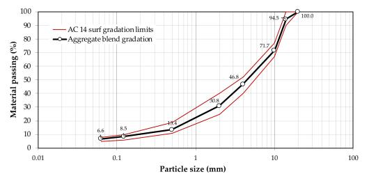
Figure 1. Grading of the aggregate's mixture and specification gradation limits.
