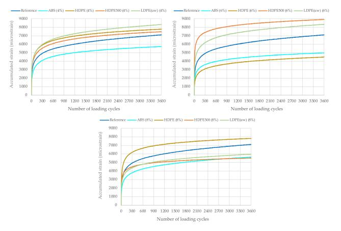
**Figure 12.** Variation of the accumulated permanent deformation measured in cyclic compression tests at 60  $^{\circ}$ C for both the reference and the asphalt concrete with different plastic wastes.
