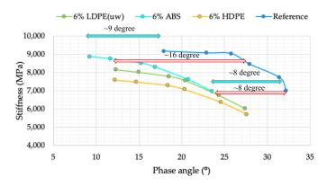
Figure 16. Black diagram derived from four-point bending tests at 20 °C.
