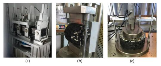
**Figure 5.** Mechanical performance tests: (**a**) four-point bending test; (**b**) indirect tensile strength test; and (**c**) cyclic compression test.
