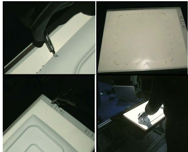
Figure 9. Programming table for product direct programming with infrared pen and augmented reality.
