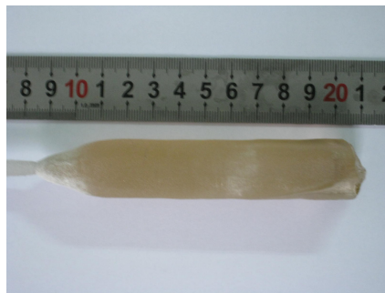
Fig. 2. Photograph of as-grown Er,Pr:GYSGG laser crystal.
