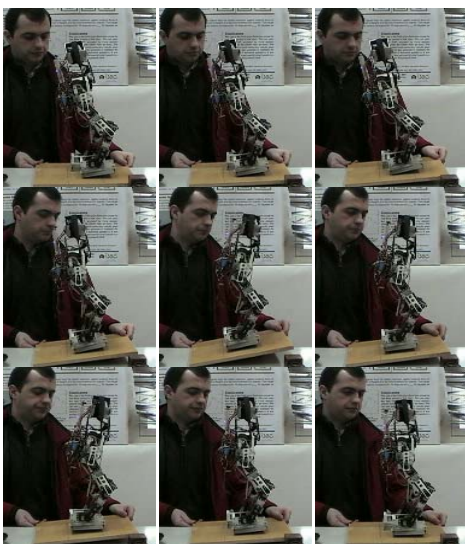
Figure 8. Snapshots of the behaviour of the robot when it is standing with one foot in the air and the slope varies from 0 to 10 degrees and 10 to 0 degrees, with the improved SVR controller
