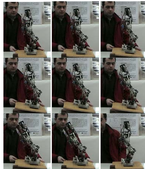
Figure 11. Snapshots of the behaviour of the robot when it is standing with one foot in the air and the slope varies from 0 to -10 degrees and -10 to 0 degrees, with the improved SVR controller
