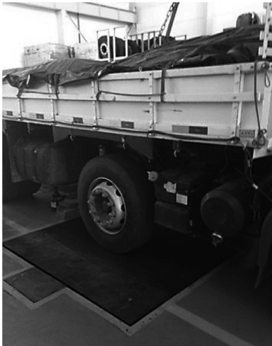
Fig. 7 – Weighting scale used for calibration.
