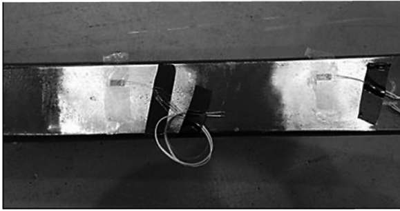
Fig. 6 – Primary suspension spring leaf-instrumentation.
