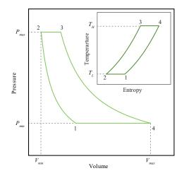
Figure 2. P-V diagram of the Ericsson cycle and T-s diagram (inset).
