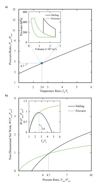
**Figure 7.** (a) Relationship between pressure and temperature ratio for equal net work output and *P*-*V* diagram of Stirling and Ericsson cycles for fixed temperature and pressure limits and maximum volume for equal net work output (inset); (b) non-dimensional net work as a function of pressure ratio and temperature ratio (inset).
