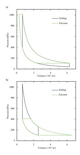
**Figure 4.** *P-V* diagrams of Stirling and Ericsson cycles for fixed mass and temperature limits with (**a**) fixed maximum pressure and volume and (**b**) fixed minimum pressure and volume.
