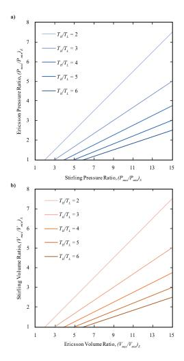
**Figure 3.** (**a**) Pressure ratio relationship and (**b**) volume ratio relationship between Stirling and Ericsson cycles, where the solid lines indicate equal net work output for equivalent mass and temperature limits.
