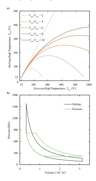
**Figure 6.** (a) High temperature relationship between Stirling and Ericsson cycles for fixed volume ratios and  $T_L = 25 \,^{\circ}$ C, with solid lines denoting equal net work output; (b) *P*-*V* diagrams of Stirling and Ericsson cycles for fixed mass, volume limits and low temperature for equal net work output.
