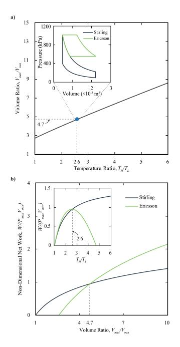
**Figure 8.** (a) Relationship between volume and temperature ratio for equal net work output and *P-V* diagram of Stirling and Ericsson cycles for fixed temperature and volume limits and maximum pressure for equal net work output (inset); (b) non-dimensional net work as a function of volume ratio and temperature ratio (inset).
