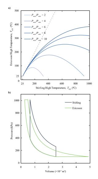
**Figure 5.** (a) High temperature relationship between Stirling and Ericsson cycles for fixed pressure ratios and  $T_L = 25 \,^{\circ}$ C, with solid lines denoting equal net work output; and (b) *P-V* diagrams of Stirling and Ericsson cycles for fixed mass, pressure limits and low temperature for equal net work output.
