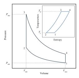
Figure 1. *P-V* diagram of the Stirling cycle and *T-s* diagram (inset).
