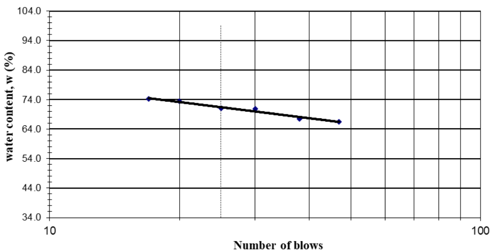
Figure 4.3: Liquid limit chart of Baixo Mondego soft soil
