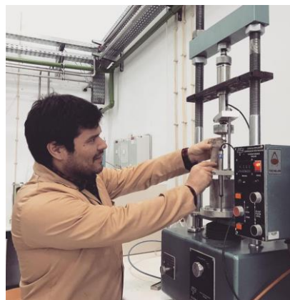
Figure 4.8: UCS Test in Wykeham Farrance equipment
