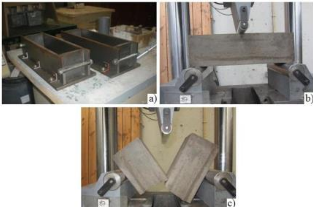
Figure 4.16: Flexural Test (adapted from Teles, 2013)
