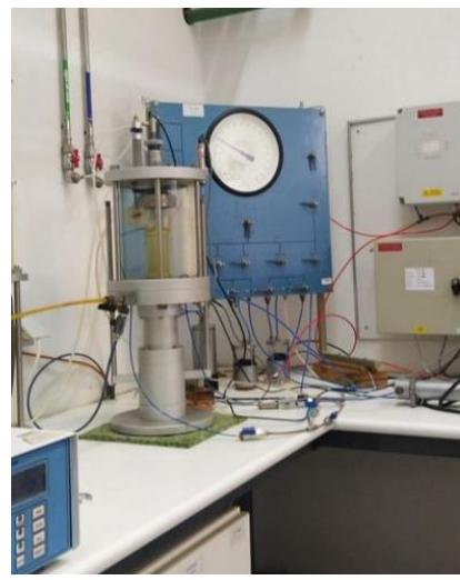
Figure 4.22: Views from a) testing operation sample b) extended view of the triaxial stress path device
