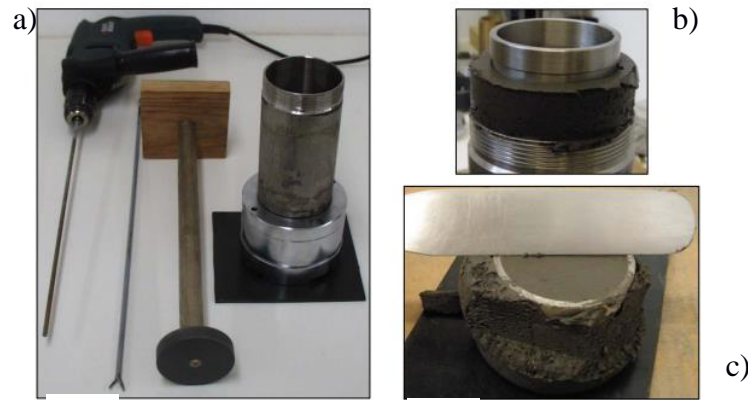
Figure 4.6: Oedometer preparations procedure (Correia, 2011)
