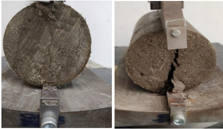
Figure 5.16: Failure mechanism imposed in a STS test
