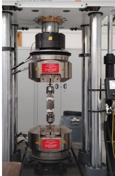
Figure 4.11: DTS Test using the universal device in mechanical lab
