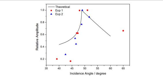
**Figure 3.** Incident angle dependence of PA waves generated by 532 nm laser pulses in independent experiments, and behavior expected from equation (1).
