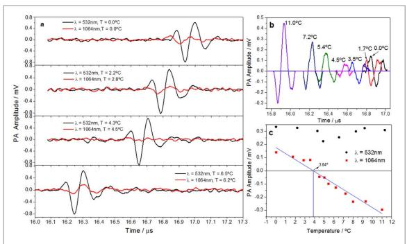
**Figure 2.** Photoacoustic (PA) waves for an angle of incidence  $\theta_i = 69.8^{\circ}$  measured with a 10 MHz transducer. (a) Temperature dependence of PA waves generated with 532 nm (black) and 1064 nm (red) laser pulses at fluence rates of 52.5 and 4.5 mJ cm<sup>-2</sup>, respectively. (b) PA waves generated with 1064 nm laser pulses at different temperatures. (c) First maximum amplitudes of PA waves generated with 532 and 1064 nm laser pulses as a function of the temperature.
