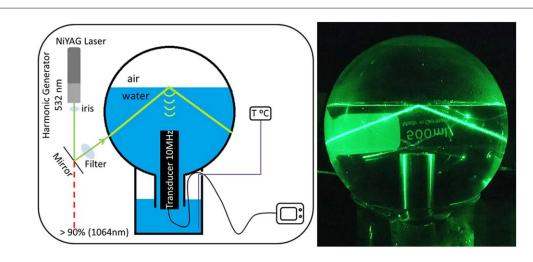
**Figure 1.** Experimental configuration. (Left) Schematic representation (filter: cutoff 1064 nm or cutoff 532 nm). (Right) Image obtained for  $\theta_i = 68.6^{\circ}$ , where total internal reflection is observed.
