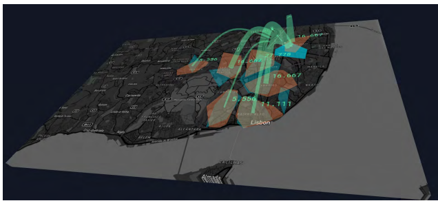
FIGURE 9. A 3D sample of trip flows from one origin area to all destination areas based on a time-dependent O-D matrix constructed for the period of 6AM - 9AM using the proposed approach, where the origin and destination areas are shown on the same map.
