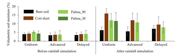
**Figure 6.** Bar graphs (mean and standard deviation of three repetitions) of volumetric soil moisture before and after rainfall simulation observed for all soil cover conditions and rainfall patterns.
