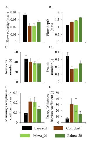
**Figure 7.** Bar graphs (mean and standard deviation of three repetitions) of hydraulic parameters of runoff estimated for all soil cover conditions and the uniform rainfall pattern: (**A**) Flow velocity, (**B**) flow depth, (**C**) Reynolds number, (**D**) Froude number, (**E**) Manning's roughness coefficient and (**F**) Darcy–Weisbach friction coefficient.
