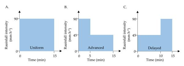
Figure 3. Rainfall patterns simulated in the experiments: (A) Uniform, (B) advanced and (C) delayed.
