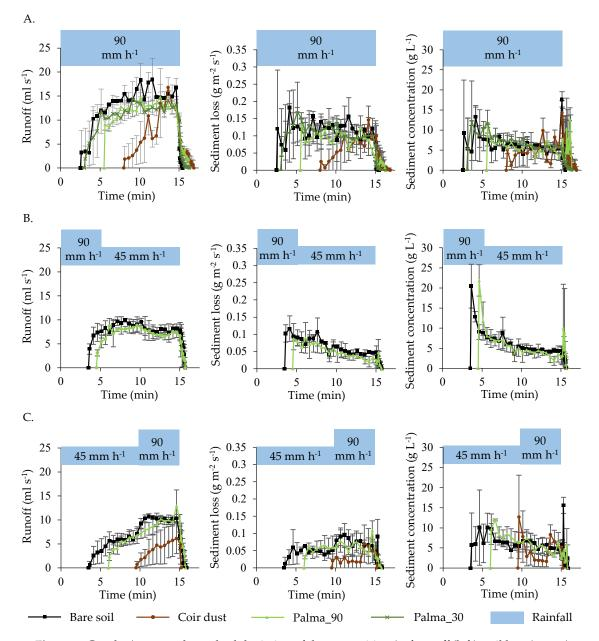
**Figure 4.** Graphs (mean and standard deviation of three repetitions) of runoff (left), soil loss (center) and sediment concentration (right) observed for all soil cover conditions and for the three rainfall patterns simulated in the experiments: (**A**) Uniform, (**B**) advanced and (**C**) delayed. No runoff and soil loss were observed for the coir dust and advanced rainfall pattern.
