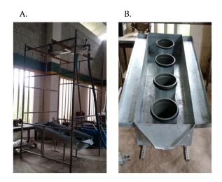
**Figure 1.** Photographs of the laboratory setup used in the experiments: (**A**) Rainfall simulator and corresponding support structure, and (**B**) Downstream view of soil flume with buffer zones.
