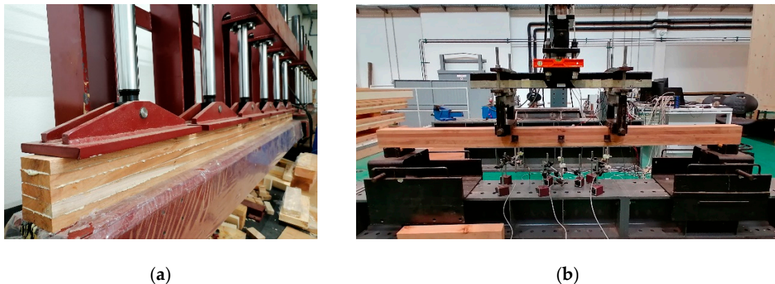
Figure 4. Blackwood glulam beam: (a) at a production stage under pressure; (b) subjected to a static MOE test.
